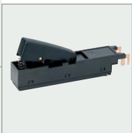
2602.5101 with passive linear potentiometer
